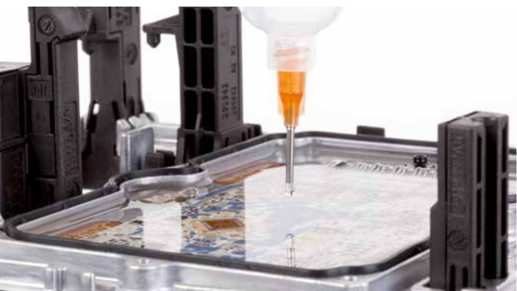
Protection against vibrations and corrosion: the amount of electronic components in cars is constantly increasing. Encapsulation makes control systems resistant to everything that impacts on vehicles: vibrations, temperature fluctuations and moisture. Image: encapsulation of an automotive electronic controller with WACKER SilGel® 612.
